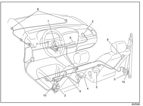
1. Driver's air bag 2. Front passenger's air bag 3. Safety belt pretensioner 4. Air bag controller (SDM) 5. Occupant classification module 6. "PASSENGER AIRBAG OFF" indicator 7. Air bag readiness light 8. Early crash sensor 9. Side air bag 10. Side air bag sensor AURORA S4U1014A The words AIR BAG will appear on the side of the front seatback closest to the door, to indicate the presence of a side impact air bag.
